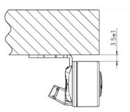
**Example 4: (Article number 914785)**The panel is mounted with a 45° bracket and placed on a tabletop with angled front.
