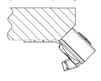
To mount the panel: Just click the panel into the bracket and it is fixed.
