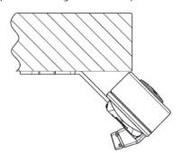
**Example 2: (Article number 914757)**The panel is mounted with a 90° bracket and placed with a distance to the tabletop.
