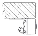
**Example 3: (Article number 914760)**The panel is mounted with a 45° bracket and placed at the edge of the tabletop.
